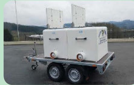
In addition we have placed particular importance on the fish transport tank's totally smooth exterior. This gives the container a pleasant appearance and makes cleaning easy, both inside and out.
