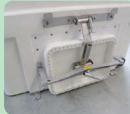
mounted standard sluce and fixing brackets
